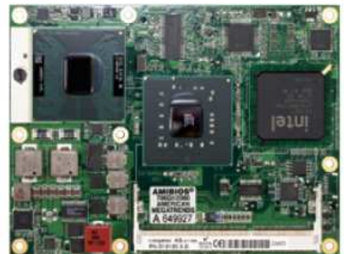
Covers Entire Range of x86 Platforms, ATOM - AMD - I7 (x86) Size: 135 x 95mm
